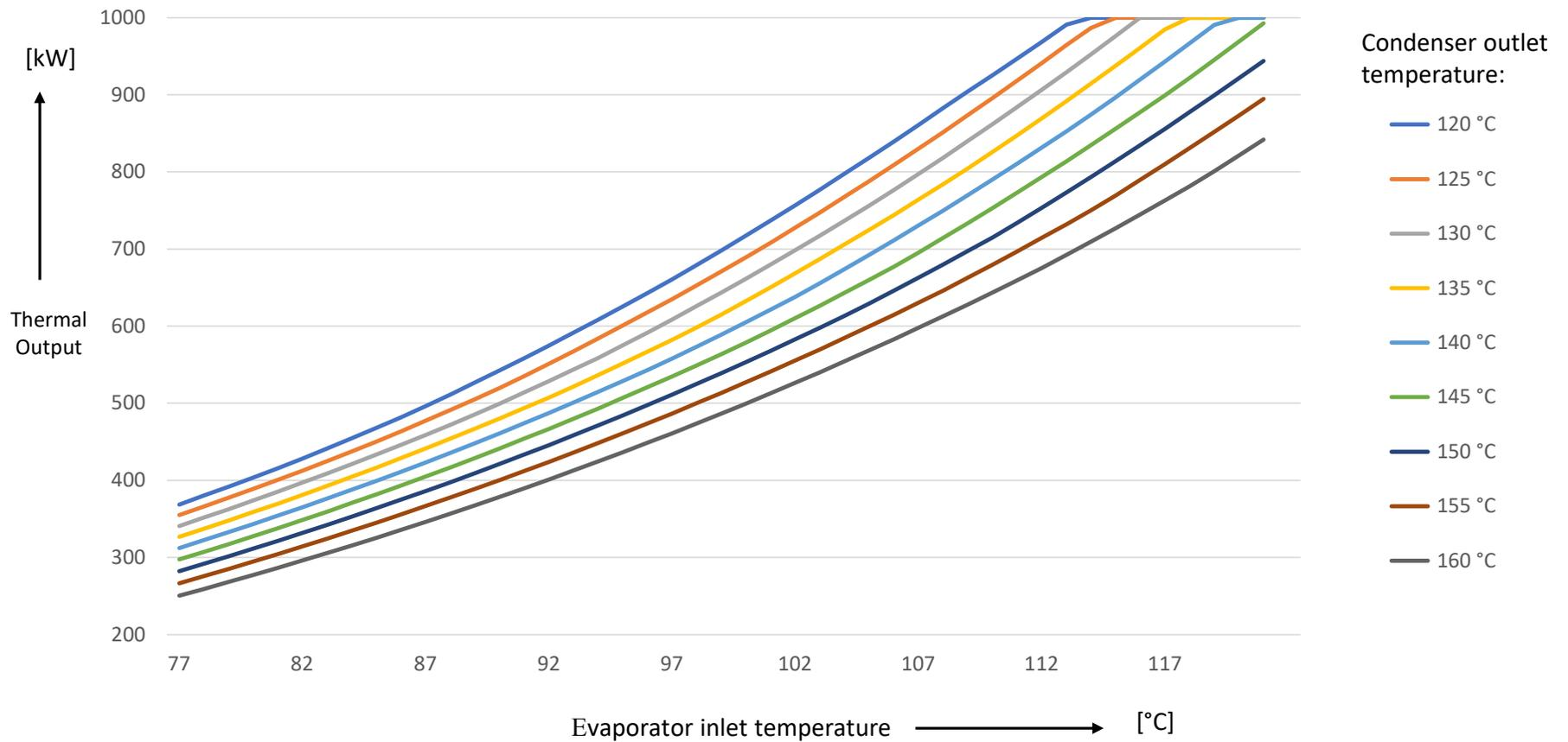
Calculated thermal output as function of the evaporator inlet temperature for different condenser outlet temperatures (R1233zd).
