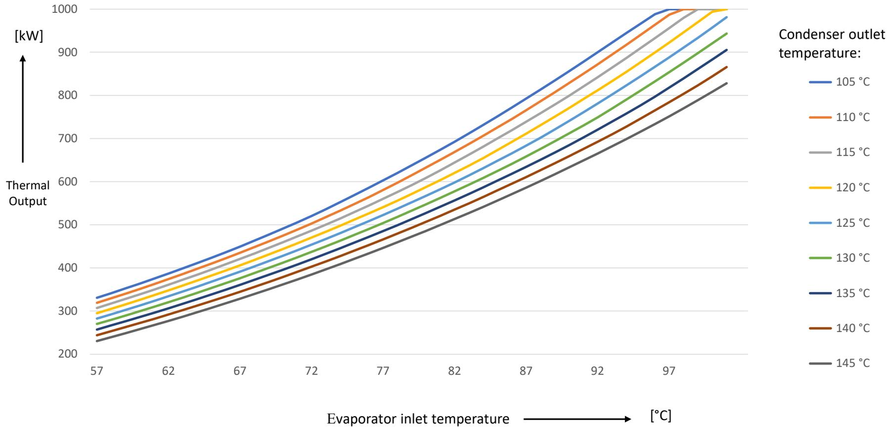
Calculated thermal output as function of the evaporator inlet temperature for different condenser outlet temperatures (R1234ze).
